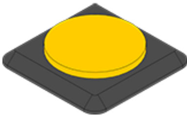
Disable Button DEPRESSED (RBB Pump Operational)
